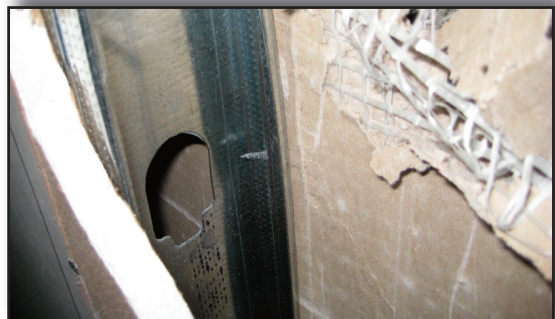
Soft body impact test using ViperStud.
